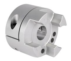
Sung-II Machinery drive coupling hub, jaw type, aluminum alloy, clamp, size 100, 30mm bore. Requires SJC-100 series spiders.
