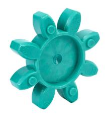
Sung-II Machinery drive coupling spider, jaw type, size 100, Hytrel, 98A durometer. For use with SJC-100C series hubs.
