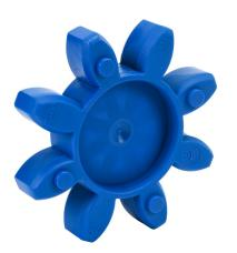
Sung-II Machinery drive coupling spider, jaw type, size 100, thermoplastic polyurethane, 98A durometer. For use with SJC-100C series hubs.
