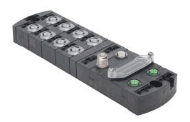
STRIDE Basic EtherNet/IP IO-Link master, (8) IO-Link capable I/O points, up to (16) discrete I/O points, IO-Link v1.1, 8A, 1A/port, IP65 and IP67.
