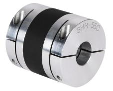
Sung-Il Machinery drive coupling, servo high gain, aluminum alloy, clamp, size 55, 19 x 24mm bore.
