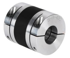
Sung-Il Machinery drive coupling, servo high gain, aluminum alloy, clamp, size 43, 19 x 20mm bore.
