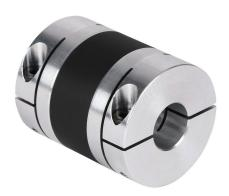
Sung-II Machinery drive coupling, servo high gain, aluminum alloy, clamp, size 38, 14 x 20mm bore.
