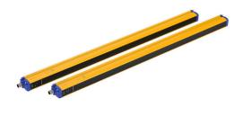
Datalogic safety light curtain, sender/receiver pair, hand protection, 24 VDC, 30mm resolution, 600mm protected height, 0.2-20m operating distance, safety category Type 4, IP65, (1) 4-pin and (1) 8-pin M12 quick-disconnect.
