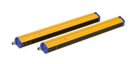
Datalogic safety light curtain, sender/receiver pair, hand protection, 24 VDC, 30mm resolution, 300mm protected height, 0.2-20m operating distance, safety category Type 4, IP65, (1) 4-pin and (1) 8-pin M12 quick-disconnect.
