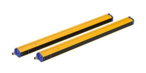
Datalogic safety light curtain, sender/receiver pair, finger protection, 24 VDC, 14mm resolution, 450mm protected height, 0.2-6m operating distance, safety category Type 4, IP65, (1) 4-pin and (1) 8-pin M12 quick-disconnect.
