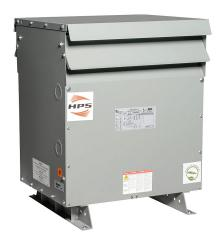
Hammond general purpose transformer, open core, 75 kVA, 3-phase, 480 VAC Delta primary, 240/120 VAC Delta (center tap) secondary, 60 Hz, NEMA 3R, floor mount.
