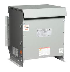
Hammond general purpose transformer, open core, 30 kVA, 3-phase, 480 VAC Delta primary, 240/120 VAC Delta (center tap) secondary, 60 Hz, NEMA 3R, floor, wall or ceiling mount.
