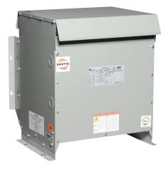
Hammond general purpose transformer, open core, 30 kVA, 3-phase, 480 VAC Delta primary, 208Y/120 VAC secondary, 60 Hz, NEMA 3R, floor, wall or ceiling mount.
