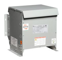
Hammond general purpose transformer, open core, 15 kVA, 3-phase, 480 VAC Delta primary, 208Y/120 VAC secondary, 60 Hz, NEMA 3R, floor, wall or ceiling mount.
