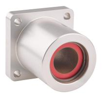
PBC Simplicity series plain bearing, PTFE bearing, 1in inside diameter, 2-13/16in overall length, self-aligning housing, closed, anodized aluminum, flanged, 0.0005in running clearance. For use with 1in diameter PBC shafts.
