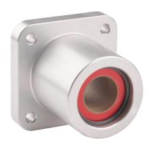
PBC Simplicity series plain bearing, PTFE bearing, 3/4in inside diameter, 2-1/16in overall length, self-aligning housing, closed, anodized aluminum, flanged, 0.0005in running clearance. For use with 3/4in diameter PBC shafts.
