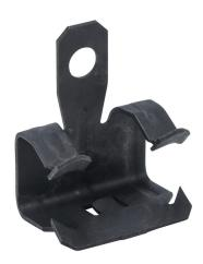
Minerallac hammer-on flange clamp, 200 lbs. Package of 100. For use with 9/16 to 3/4in flanges and 1/4in hole.
