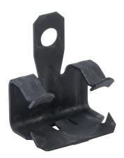
Minerallac hammer-on flange clamp, 200 lbs. Package of 25. For use with 9/16 to 3/4in flanges and 1/4in hole.
