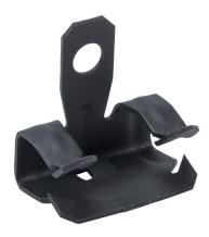
Minerallac hammer-on flange clamp, 200 lbs. Package of 100. For use with 5/16 to 1/2in flanges and 1/4in hole.
