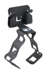
Minerallac hammer-on flange clamp conduit hanger assembly, spring clip, back mount, 25 lbs, UL Type UL 2239. Package of 100. For use with 1/8 to 1/4in flanges and 1/2 or 3/4in conduit.
