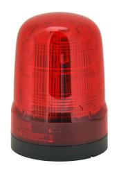
Patlite SF series LED industrial signal beacon, 100mm, red, (22) selectable flashing and rotating patterns, IP66, NEMA 4X/13, base mount, 100-240 VAC.
