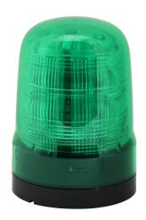
Patlite SF series LED industrial signal beacon, 100mm, green, (22) selectable flashing and rotating patterns, IP66, NEMA 4X/13, base mount, 100-240 VAC.
