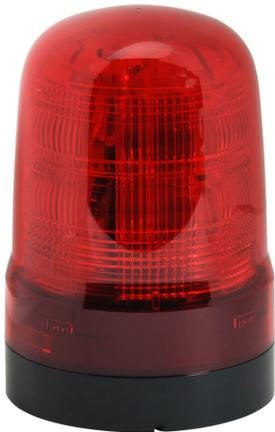
Patlite SF series LED audible-visual signal beacon, 88 dB at 1m, continuous tone(s), (22) selectable flashing and rotating patterns, red, 100mm, 100-240 VAC, IP66, NEMA 4X/13, push-in terminal.
