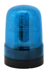
Patlite SF series LED audible-visual signal beacon, 88 dB at 1m, continuous tone(s), (22) selectable flashing and rotating patterns, blue, 100mm, 100-240 VAC, IP66, NEMA 4X/13, push-in terminal.
