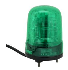
Patlite SF series LED industrial signal beacon, 100mm, green, (22) selectable flashing and rotating patterns, IP23, base mount, 100-240 VAC. IP65 when used with SZW-103 rubber gasket.
