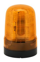
Patlite SF series LED audible-visual signal beacon, 88 dB at 1m, continuous tone(s), (22) selectable flashing and rotating patterns, amber, 100mm, 12-24 VDC, IP66, NEMA 4X/13, push-in terminal.
