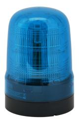
Patlite SF series LED audible-visual signal beacon, 88 dB at 1m, continuous tone(s), (22) selectable flashing and rotating patterns, blue, 100mm, 12-24 VDC, IP66, NEMA 4X/13, push-in terminal.
