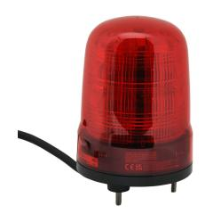
Patlite SF series LED industrial signal beacon, 100mm, red, (22) selectable flashing and rotating patterns, IP23, base mount, 12-24 VDC. IP65 when used with SZW-103 rubber gasket.
