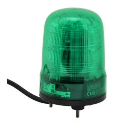
Patlite SF series LED industrial signal beacon, 100mm, green, (22) selectable flashing and rotating patterns, IP23, base mount, 12-24 VDC. IP65 when used with SZW-103 rubber gasket.
