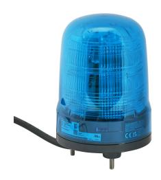
Patlite SF series LED industrial signal beacon, 100mm, blue, (22) selectable flashing and rotating patterns, IP23, base mount, 12-24 VDC. IP65 when used with SZW-103 rubber gasket.
