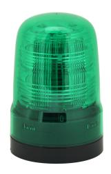
Patlite SF series LED industrial signal beacon, 80mm, green, (22) selectable flashing and rotating patterns, IP66, NEMA 4X/13, base mount, 100-240 VAC.
