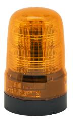
Patlite SF series LED audible-visual signal beacon, 86 dB at 1m, continuous tone(s), (22) selectable flashing and rotating patterns, amber, 80mm, 100-240 VAC, IP66, NEMA 4X/13, push-in terminal.
