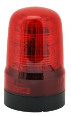
Patlite SF series LED audible-visual signal beacon, 86 dB at 1m, continuous tone(s), (22) selectable flashing and rotating patterns, red, 80mm, 100-240 VAC, IP66, NEMA 4X/13, push-in terminal.
