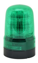
Patlite SF series LED audible-visual signal beacon, 86 dB at 1m, continuous tone(s), (22) selectable flashing and rotating patterns, green, 80mm, 100-240 VAC, IP66, NEMA 4X/13, push-in terminal.
