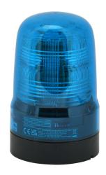
Patlite SF series LED audible-visual signal beacon, 86 dB at 1m, continuous tone(s), (22) selectable flashing and rotating patterns, blue, 80mm, 100-240 VAC, IP66, NEMA 4X/13, push-in terminal.
