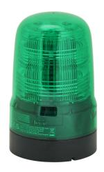
Patlite SF series LED audible-visual signal beacon, 86 dB at 1m, continuous tone(s), (22) selectable flashing and rotating patterns, green, 80mm, 12-24 VDC, IP66, NEMA 4X/13, push-in terminal.
