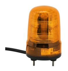
Patlite SF series LED industrial signal beacon, 80mm, amber, (22) selectable flashing and rotating patterns, IP23, base mount, 12-24 VDC. IP65 when used with SZW-102 rubber gasket.
