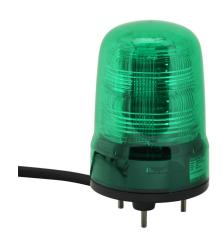
Patlite SF series LED industrial signal beacon, 80mm, green, (22) selectable flashing and rotating patterns, IP23, base mount, 12-24 VDC. IP65 when used with SZW-102 rubber gasket.
