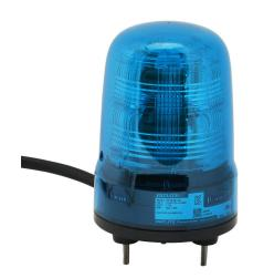
Patlite SF series LED industrial signal beacon, 80mm, blue, (22) selectable flashing and rotating patterns, IP23, base mount, 12-24 VDC. IP65 when used with SZW-102 rubber gasket.
