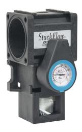
CITO StackFlow modular manual valve, 2-way, 2-position, glass-filled nylon body, stackable, Cv=21.3. FT-200 temperature gauge and RA-3903 high-flow turbine included.
