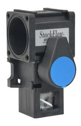
CITO StackFlow modular manual valve, 2-way, 2-position, glass-filled nylon body, stackable, Cv=21.3. RA-3903 high-flow turbine included.
