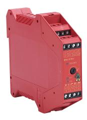
IDEM safety relay extension module, release delay, 0 to 30 seconds, 24 VAC/VDC, (3) N.O. time delay safety output(s), (1) N.C. time delay monitoring output(s), fixed screw terminals.
