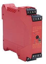
IDEM safety relay extension module, release delay, 0 to 30 seconds, 24 VAC/VDC, (3) N.O. time delay safety output(s), (1) N.C. time delay monitoring output(s), pluggable screw terminals.
