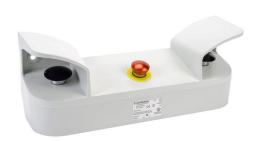
Schmersal control panel, two-hand safety, plastic, (1) Estop, (2) momentary pushbuttons, mushroom, red/black/black, (2) N.O/(2) N.C. and (1) N.O./(1) N.C. and (1) N.O./(1) N.C. contact(s), blank legend plate(s).
