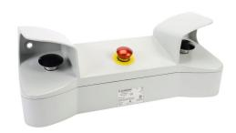
Schmersal control panel, two-hand safety, die-cast aluminum, (1) Estop, (2) momentary pushbuttons, mushroom, red/black/black, (2) N.O/(2) N.C. and (1) N.O./(1) N.C. and (1) N.O./(1) N.C. contact(s), blank legend plate(s).
