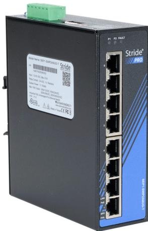
STRIDE PRO industrial unmanaged+ PoE+ switch, IEEE 802.3af/at, 240W, 8 ports, (8) PoE+ Gigabit (RJ45) port(s), 12–55 VDC nominal input, -40 to +75 °C, 35mm DIN rail or panel mount.
