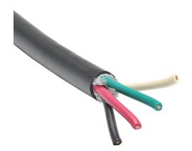
Southwire portable cord, unshielded, SEOOW, 600V, 4 conductors (includes ground), 18 AWG, TPE conductor insulation material, black, white, red and green, TPE jacket, black, cut to length.
