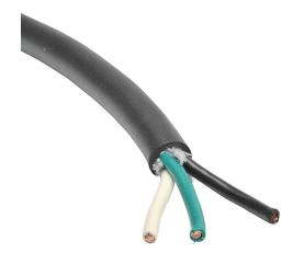
Southwire portable cord, unshielded, SEOOW, 600V, 3 conductors (includes ground), 18 AWG, TPE conductor insulation material, black, white and green, TPE jacket, black, cut to length.
