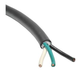
Southwire portable cord, unshielded, SEOOW, 600V, 3 conductors (includes ground), 18 AWG, TPE conductor insulation material, black, white and green, TPE jacket, black, cut to length.
