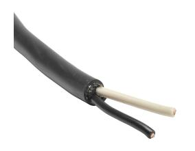
Southwire portable cord, unshielded, SEOOW, 600V, 2 conductors, 18 AWG, TPE conductor insulation material, black and white, TPE jacket, black, cut to length.
