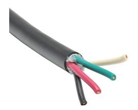
Southwire portable cord, unshielded, SEOOW, 600V, 4 conductors (includes ground), 16 AWG, TPE conductor insulation material, black, white, red and green, TPE jacket, black, cut to length.
